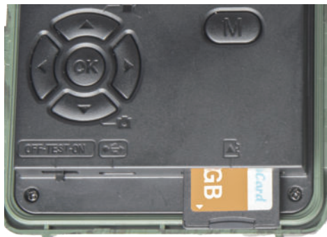
Figure 7: Inserting the SD Card
