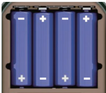
Figure 6: Loading the Batteries
