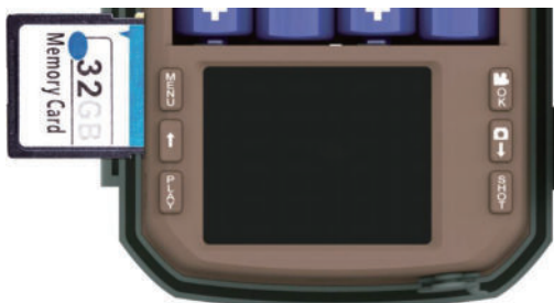
Figure 7: Inserting the SD Card
